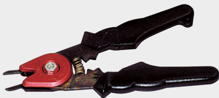
Designation Art. no. MIG/MAG special gun Size 1, for 12-15 mm tips 1091000 Size 2, for 15-18 mm tips 1092000 ▶ Fast and dimensionally true cutting of the filler wire ▶ Time-saving cleaning and honing of the shield gas tip, and loosening and tightening the contact tip
